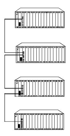
Figure 2-4. Serial Configuration Using 10BASE-FL Modules
